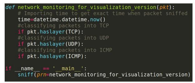
Fig 4: Classifying packets into TCP, UDP and ICMP
